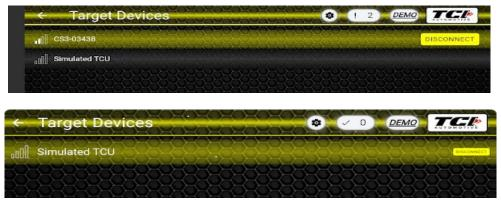
E. Wait for the connection. When connected, a check mark will appear and a "0" for no trouble codes. NOTE: Carbureted applications with standalone TPS may see (I) DTC code for TPS calibration. This is normal and should clear once the TPS Calibration step is complete.
